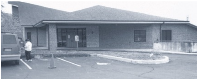
Image 10: By placing an orange cone in the adjacent parking stall, this polling place now meets van accessibility parking requirements.
