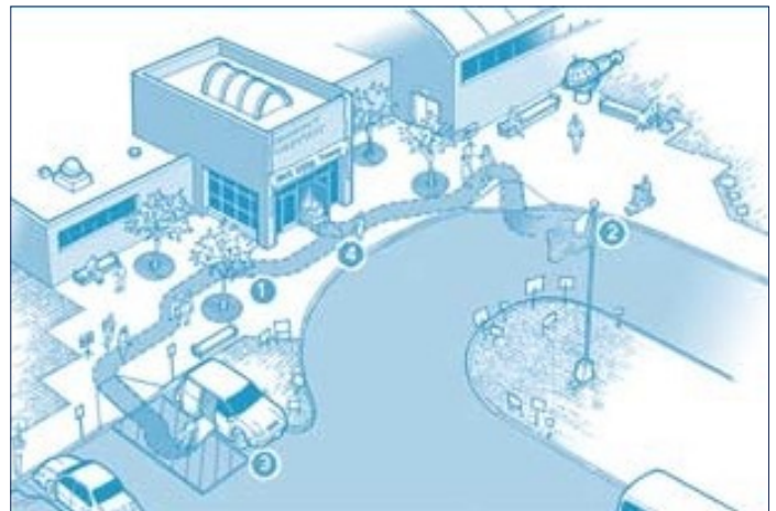
Image 11: An accessible entrance to a voting location with accessible parking and an accessible drop-off area. 1 – Accessible route. 2 – Accessible drop-off area. 3 – Accessible parking with van-accessible parking space. 4 – Accessible entrance to the voting location.
