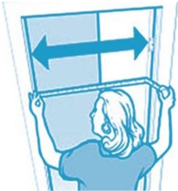
Image 5: Measuring the clear opening from the face of the doorstop on the frame to the face of the open door.
