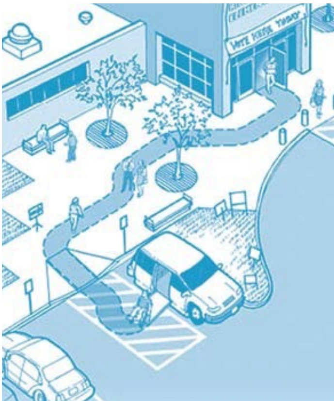
Image 7: Accessible route from the parking lot to the voting location.
