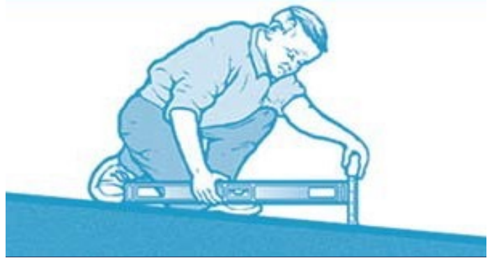
Image 3: Measuring a slope using a 24-inch level and tape measure.
