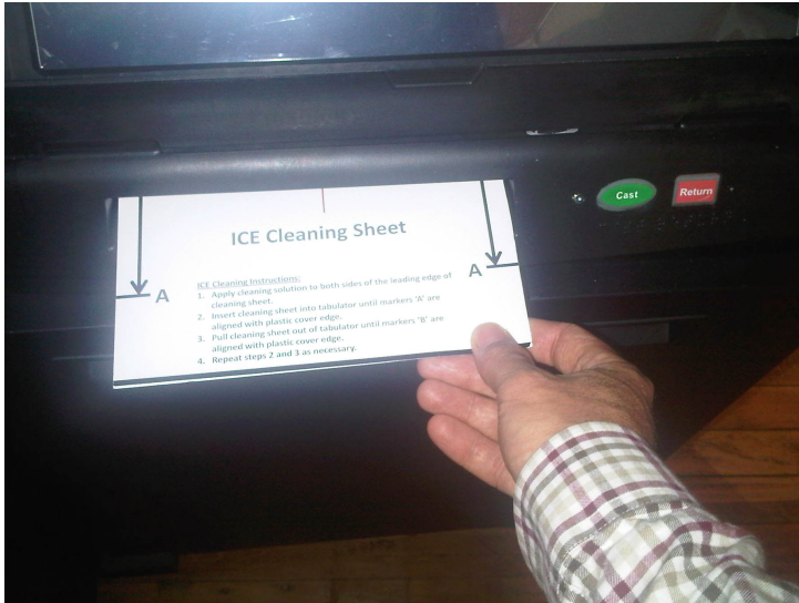
Figure 5.3: Inserting ICE Cleaning Sheet
