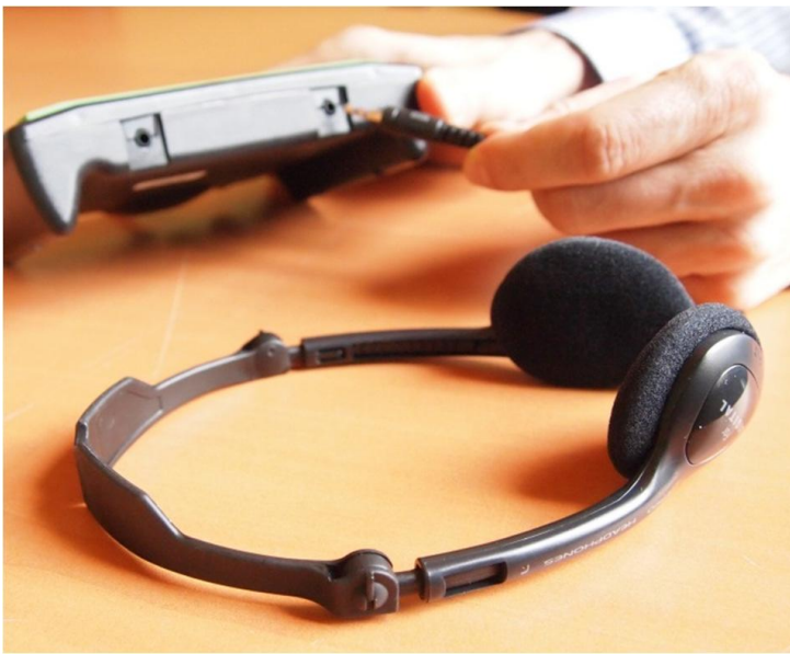
Figure 5.7: Connect the headphones to the headphone jack at the bottom of the ATI.
